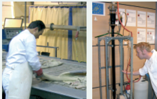
Pieces of meat are cut from the rawhides (left photo) and the biogas potential of the meat offal is thoroughly examined in the experimental setup at the laboratory at the tannery's Research and Development Centre (right photo).
